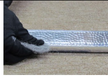
8. Scratch=Pulls a bit of the base coat to the surface of the moulding
