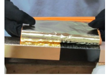
6. Gilding=Hand laid foil placed on moulding for final color
