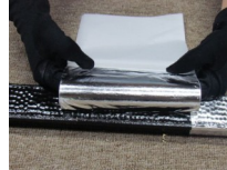
6. Gilding=Hand laid foil placed on moulding for final color
