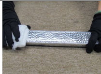
7. Leaf Polish=Smooths out and adheres foil to the moulding
