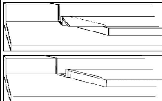
Wooden strips support Rabbetspace in chopper or saw when cutting. The wooden strips are available in four sizes to match the four different Rabbetspace depths.
